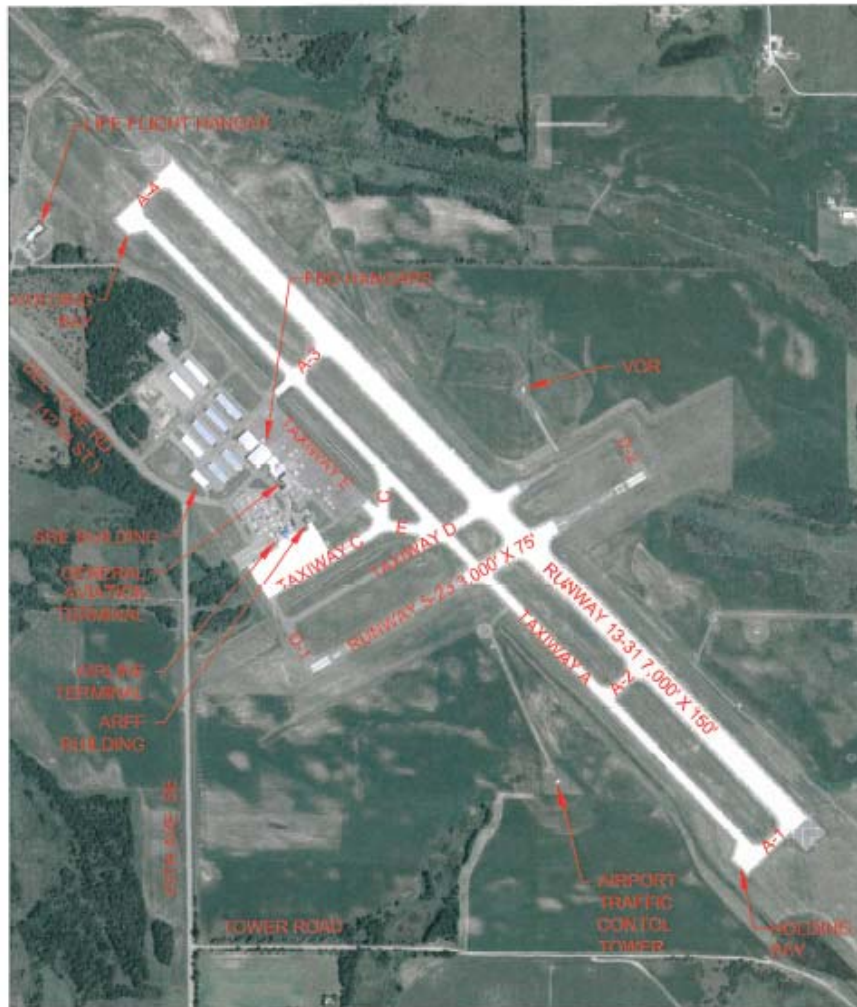
Figure 9-2 St. Cloud Regional Airport Existing Layout
